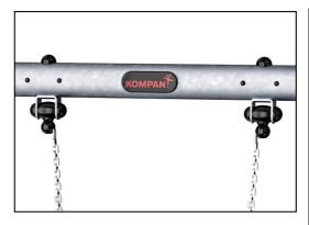
The swing hangers are made of high quality UV-stabalised nylon (PA6) housing with integrated lifetime sealed ball bearings. The height adjustable chains are fixed by a stainless steel hook with theft proof snake-eye bolt in a turn able anti twist housing. All seats with two chain fixation are available with either standard or anti-wrap suspension.
