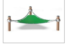
Corocord membranes consist of friction-proof rubberized material of conveyor belt quality with excellent UV resistance. Tested and compliant with REACH requirements for PAH. Embedded is a four-layered armouring made of woven polyester. The armouring and the two surface layers result in a total thickness of 7.5 mm.
