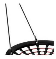
Ropes are made of UV-stabilised PA with inner steel cable reinforcement. The rope is induction treated to create a secure connection between steel and rope, which leads to excellent wear resistance.
