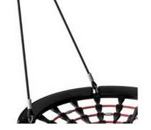
Ropes are made of UV-stabilised PA with inner steel cable reinforcement. The rope is induction treated to create a secure connection between steel and rope, which leads to excellent wear resistance.
