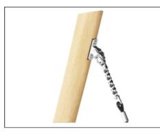
The swing hangers are made of stainless steel brackets and can move over two axis. The flange bearings are silicone enriched to make the suspension maintenance free. The connection to the rope is made with stainless steel chain.
