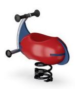
The seat is made of recyclable PE and molded in one piece with a minimum 5mm wall thickness. PE has high impact resistance across a wide temperature span which ensures vandal resistance in all locations.
