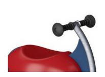
Handles are made with a molded PP insert and an outer layer of soft TPV rubber. The handles are attached to the pipe with a galvanized steel inlay to ensure strength and durability.
