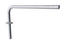
Handrail intended as grips during exercises are made of hot-dip galvanised steel ø38mm, a great diameter for a good grip and to support the wrist. The height of the handrail is 940mm from the top of the HPL plate. The distance between the rails is 900mm.
