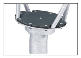
Upper plate is made of Ekogrip® panel that consist of a 15mm thick PE base with 3 mm top-layer of soft rubber with a non-skid effect.
