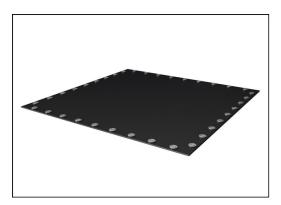
The jumping membranes are made of 6.0mm thick EP Ethylene-Propylene conveyor belt with polyester polyamide fabric carcass. Spring fixations are reinforced with steel bushings and washers on both sides. The membrane is ozone resistant and equipped with 5 center placed water drain holes.
