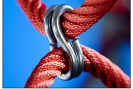
Corocord 'S' clamps are used as universal connections in Corocord products. 8mm stainless steel rods with rounded edges are pressed around the ropes with a special hydraulic press, making them the ideal connector: safe, durable and vandalism-proof, all while allowing the typical movement of rope play structures.
