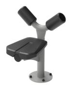
The seat is made of Polyurethane Rubber and has a steel insert plate that is electrogalvanized. The steel plate connects the seat to the frame. This construction makes the seat extremely durable against wear & tear and still very comfortable for a great user experience. The seat is positioned at a height of 46 cm, a comfortable height that makes the transfer from a wheelchair easy.
