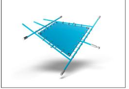
Corocord membranes consist of friction-proof rubberized material of conveyor belt quality with excellent UV resistance. Tested and compliant with REACH requirements for PAH. Embedded is a four-layered armouring made of woven polyester. The armouring and the two surface layers result in a total thickness of 8 mm.
