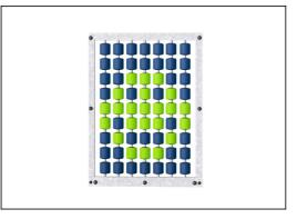
The two colored turnable rollers are made of high quality UV stabilized and reinforced nylon (PA). The rollers are assembled on vertical steel pipes in a welded frame. All steel parts are hot dip galvanized.
