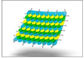
Colorful "Dragon Scale" made of friction-proof rubberized membrane of conveyor belt quality with excellent UV resistance. Embedded are two layers of galvanized steel wire armoring, making the membrane extremely durable.
