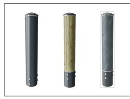
Main posts with hot dip galvanized steel footing are available in different materials: Pressure impregnated pine wood posts. Pre-galvanized inside and outside with powder coated top finish steel posts. Lead free aluminum with color anodized top finish. Greenline TexMade posts of 95% post-consumer recycled PE and textile waste.
