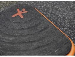
The surface is produced of recycled SBR
