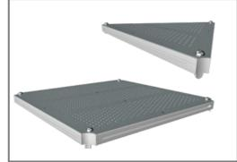
All decks are made of perforated low carbon steel plates supported by aluminum profiles with no unsupported area larger than four square feet. After metallization the decks are coated with a polyurea non-slip surface which provides extremely good wear and tear resistance.
