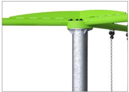
Center post is hot-dip galvanised in dimension  $\emptyset$ 159 x 4 mm. Horizontal beams are hot-dip galvanised and powder coated in dimension  $\emptyset$ 76,1 x 3,6 mm.
