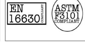
All KOMPAN fitness products are compliant with the ASTM F3101 & EN16630 Outdoor Fitness Standards. Load tests are performed as a static test by adding dynamic factors as well as safety factors to the specified load of 78kg per user. A product intended for 1 user is loaded with 420kg.
