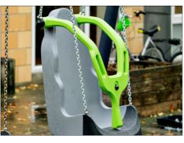
The Harness is made of molded recyclable polyethylene (PE) made from 33% post consumer materials. The harness utilizes a stainless-steel torsion spring which makes the harness stay in in all position to secure easier entry and exit of users. the harness lock is designed with a one-handed operation slider made from stainless steel.
