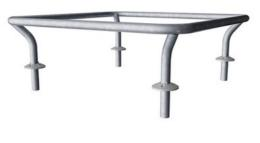
Handrail intended as grips during exercises are made of hot-dip galvanized steel ø38mm, a great diameter for a good grip and to support the wrist. The height of the handrail is 940mm from the top of the HPL plate. The distance between the rails is 900mm.
