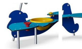
Play activities like the Funnel are made of injection molded high quality nylon (PA6). PA6 has good wearing and impact strength and is UV stabilized. Yellow basin is made from UV-stabilized PC with a thickness of 3 mm. The basin can be lifted up for emptying. The basin is fixed to the structure by a steel chain to prevent removal.
