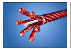
Corocord ropes of UV-stabilized PES rope strands with inner steel cable reinforcement. The polyester yarn is made from +95% postconsumer materials and is inductively melted onto each strand. PES has high strength with excellent resistance to abrasion and UV radiation. The ropes are connected by stainless steel S-Clamps which are pressed around the rope which results in a durable and vandalism solution.
