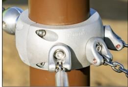
Corocord smart clamps are carefully designed in every detail to ensure superior flexibility in high quality aluminum material. The smart clamps are attached around the posts with four steel bolts. Not used attachment points are closed with PA caps.
