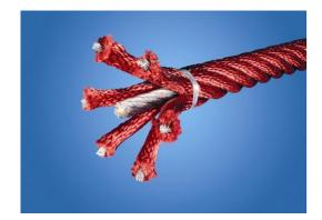
Saturn ropes has six-stranded steel wires and a steel wire core. Each strand is tightly wrapped with PES yarn, which is melted onto each individual strand and made from +95% Postconsumer Materials. After initial friction has removed the surface fibres, a harder PES coating remains to protect each strand, making the ropes highly wear- and vandalism-resistant.
