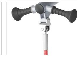
The two angled top handles are made of a moulded PP insert with an outer soft layer of TPV rubber. The handle is attached to the pipe with a galvanised steel inlay to ensure strength and durability.
