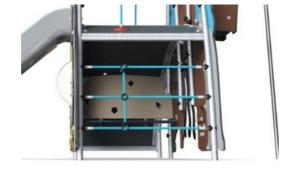
Climbing nets are made of UV-stabilised PP rope with inner steel cable reinforcement. The rope is induction treated to obtain maximum fixation between steel and rope, which provides excellent wear and tear resistance. All rope connectors are made of 100% recyclable PA material.
