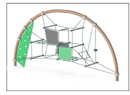
The bent arches are holding the tensioned net structure without additional disturbing fasteners. Therefore, the arches are produced from high degree stainless steel to allow movement of the net on the surface of the steel arches. The surface is then treated to create a shiny finish.
