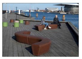
The Loops modular elements are made of rotation-molded polyethylene (PE) with a 6-7mm thickness. The Loops are UV-resistant, have excellent impact strength, and are usable within a large temperature span.
