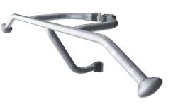
The frame of the leg lift is made from Ø38 x 2mm HDG steel tube. The support plates are made from 15mm Ekogrip®, a 15 mm PE plate with a 3 mm top-layer of thermoplastic rubber with non-skid effect. The arm supports are 110 x 195mm, 580mm apart, and 1315mm above ground. The back support is 335 x 500mm. The opening in the back is 30 x 350mm. The pull up bar is made from Ø32 mm HDG steel bar. The bar is 1080mm wide and 2300mm above ground
