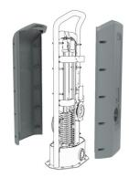
The cover protects all the moving parts from vandalism and entrapments. The cover is made of 5mm rotomolded LLDPE, Linear low-density polyethylene, with excellent impact strength and usable within a large temperature span.
