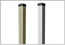
The main tower posts are available in two types of material: European pine wood posts pressure impregnated Class 3 with Tanalith E preservative, or aluminium with an anodised surface treatment.
