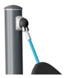
Unique KOMPAN swivel suspensions allowing for both swinging and rocking movement of the hammock. The inside housing is made of stainless steel and both the bushing and bearing rod of brass alloy. The outside cover is made of soft TPV rubber and the entire swivel is attached to the steel post by an aluminum connector.
