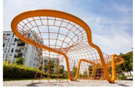
The steel surface of these bended steel pipes are wet painted with one basic layer and one top layer of lead free colour material. The paint has excellent corrosion resistance and can be easily maintained.
