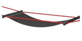
Corocord membranes consist of friction-proof rubberized material of conveyor belt quality with excellent UV resistance. Tested and compliant with REACH requirements for PAH. Embedded is a four-layered armouring made of woven polyester. The armouring and the two surface layers result in a total thickness of 7.5 mm.
