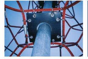
Corocord membranes consist of friction-proof rubberised material of conveyor belt quality with excellent UV resistance. Tested and compliant with REACH requirements for PAH. Embedded is a four-layered armouring made of woven polyester. The armouring and the two surface layers result in a total thickness of 7.5 mm.
