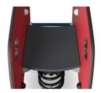
Seat is made of Ekogrip™ panel that consist of a 15mm thick PE base with 3 mm top-layer of soft rubber with a non-skid effect.
