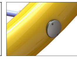
The rope is fixed to the large steel pipe by a unique KOMPAN designed tightening solution. It consists of inner and outer nylon (PA6) bushings that guides the rope to an outside threaded aluminum part that tighten the rope.
