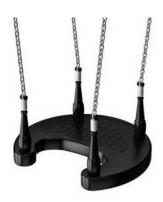
KOMPAN's curved toddler seat is made with an insert of 21.25 mm thick plywood from alder and pine wood. The outside layer is moulded in UV stabilised PUR which retains its properties within temperature ranges of -30°C to 60°C
