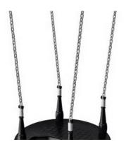
The double steel yoke suspension provides the unique parallel movement of the seat. The swing hangers are manufactured with high-quality UV stabilised nylon (PA6) which include integrated lifetime sealed ball bearings. The adjustable height chains are fixed by a stainless steel hook, snake eye bolts which are then encased within anti-twist and vandalism proof housing units.
