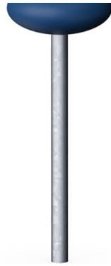
The tube of the Grasshopper is made of a Ø48,3 x 2,9mm, hot dip galvanized steel tube. The top seat is connected with a M12 bolt and covered by a PE top cap.
