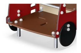
Seats are made of 22 mm thick plywood made from alder and pine wood. Both sides are covered by 2 layers of phenolic film with anti slip net pattern. All cutting edges are sealed with paint to ensure long lifetime.
