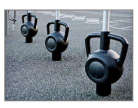
The tubes on which the magnetic bells move are ø40mm, made of grade AW 6082-T6 aluminium and have an anodized layer of 20µm. The tube has a full steel core for structural integrity.
