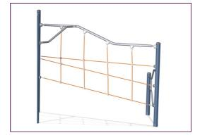
ELEMENTS ropes have six-stranded steel wires and a steel wire core. Each strand is tightly wrapped with PES yarn, which is melted onto each individual strand. After initial friction has removed the surface fibres, a harder PES coating remains to protect each strand, making the ropes highly wear and vandalism resistant.
