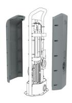
The cover protects all the moving parts from vandalism and entrapments. The cover is made of 5mm rotomolded LLDPE, Linear low-density polyethylene, with excellent impact strength and usable within a large temperature span.
