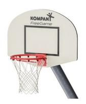
The basketball hoop is made from hot dipped galvanized steel with a powder coated finish. The net is made from Ø4 chain links made from s235 Galvanized steel or stainless-steel chains which meet the requirements in ISO1434-ISO1435 and DIN766. The chains have a circumference of ~Ø30cm at the bottom and ~Ø50cm at the top.
