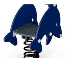
Seat is made of Ekogrip<sup>™</sup> panel that consist of a 15mm thick PE base with 3 mm top-layer of soft rubber with a non-skid effect.
