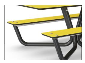
All boards are made of High Pressure Laminate HPL with a thickness of 17.8mm according to EN 438-6 and has a nonskid surface texture. The multilayer construction makes the boards durable and suitable for outdoor use with a high UV stability and high resistance to impacts, scratches, fire, water and humidity.
