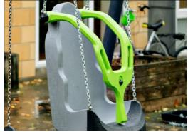
The Harness is made of molded recyclable polyethylene (PE) made from 33% post consumer materials. The harness utilizes a stainless-steel torsion spring which makes the harness stay in in all position to secure easier entry and exit of users. the harness lock is designed with a one-handed operation slider made from stainless steel.
