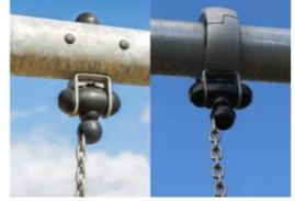
The swing hangers are made of high quality UVstabalised nylon (PA6) housing with integrated lifetime sealed ball bearings. The height adjustable chains are fixed by a stainless steel hook with theft proof snake-eye bolt in a turn able anti twist housing. All seats with two chain fixation are available with either standard or anti-wrap suspension.
