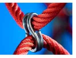
Corocord 'S' clamps are used as universal connections in Corocord products. 8mm stainless steel rods with rounded edges are pressed around the ropes with a special hydraulic press, making them the ideal connector: safe, durable and vandalism-proof, all while allowing the typical movement of rope play structures.
