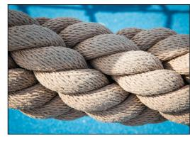
The PP rope in coconut style has a diameter of 150 mm. The internal steel wire core has thimbles at both ends, which serve as attachments for the rope to existing connecting elements.
