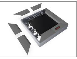
As a unique feature the SBR tiles can be removed for cleaning and service. By loosen six screws the SBR tile can be lifted up to open and gain access to the springs (see instruction on KOMPAN Master). If customized colors of the surfacing is requested all jumpers can be ordered with steel plates suitable for in situ surfacing in preferred color. For in situ installations there is no service opening option.
