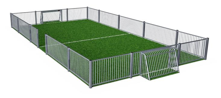
The distance between the vertical tubes is small enough to keep even small balls, such as field hockey balls, inside the pitch at all times. By embedding the tubes into the steel frame we have created an extremely vandalism proof Panel that can be placed in the toughest of neighborhoods. The galvanized tubes almost disappear from a distance. This transparent
